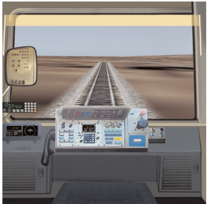
control x-train with the central console (middle center), the radio/compass unit (lower left), the GPS (middle left), and the rear wall-mounted switchboard (see mirror, upper left)
