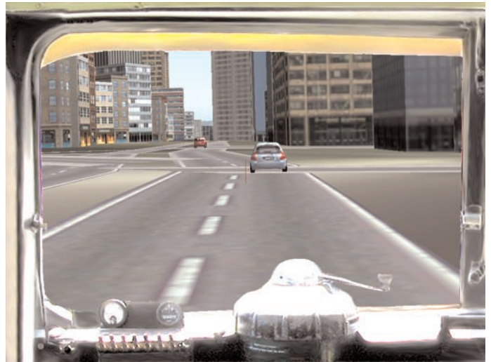
control x-train sfmuni with the main console (lower left), the throttle (right knob), and the air brakes (middle)
